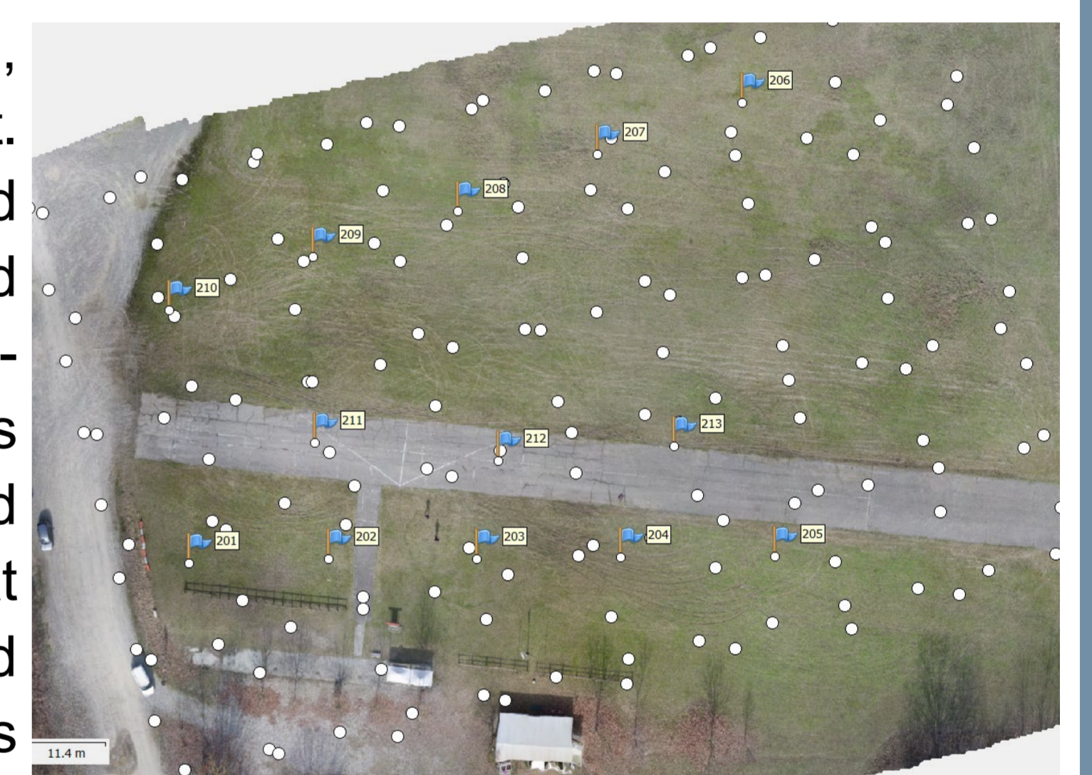
Fig. 7: Survey area of the test site. Blue flags are the GCPs and white dots are the positions of all the camera in the photogrammetric blocks.
