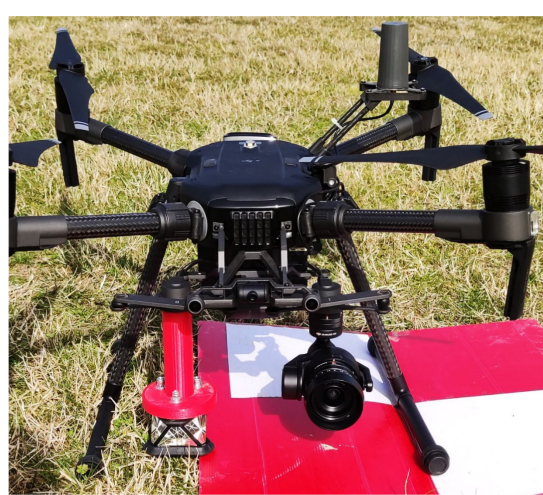
Fig. 1: The DJI Matrice 210 V2 with a Zenmuse X5S camera and the Emlid Reach M GNSS receiver mounted on the drone.
